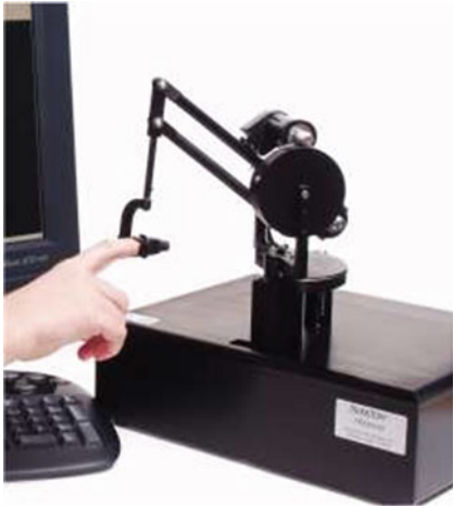
Locally Weighted Regression for Control, Fig. 5 SensAble Phantom haptic robotic arm
