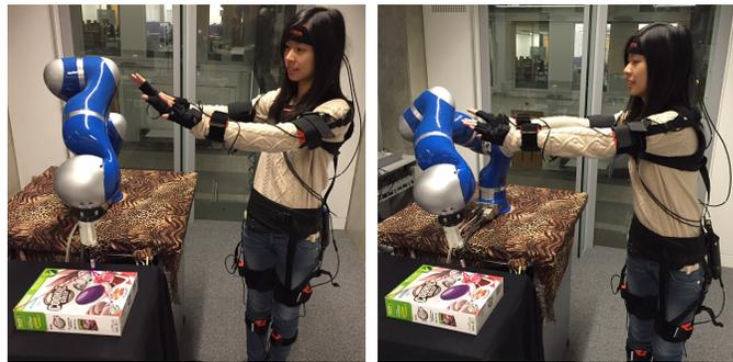
Figure 1: Robot-human close interaction. Left figure shows the robot's original motion, the right figure shows the adapted motion when human subject pushes her hands to block the original trajectory.
