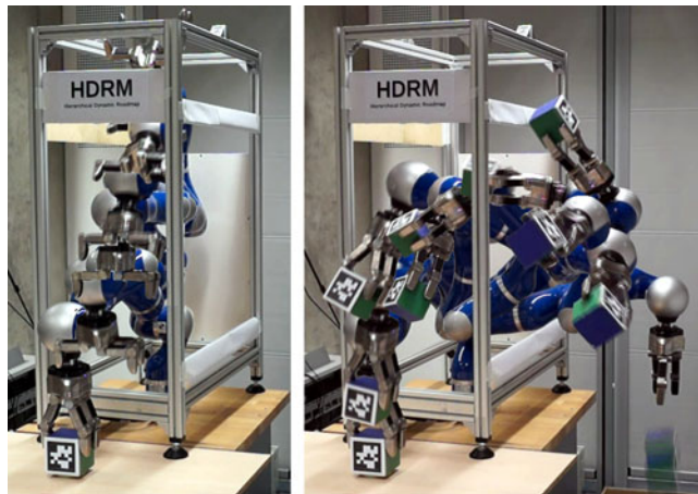
Fig. 1. The 7-DoF KUKA LWR robot with a SCHUNK Dexterous Hand operating inside a cage. Left: grasping the target from upright posture; right: dropping the object to the side.
