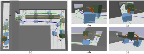
Fig. 4. Experiment 1: (a) Keyframes of multi-robot collaborative transportation, (b) and (c) are configurations that pass through the interior door, (d) and (e) are configurations that pass through narrow passage and allow obstacle through robot team.
