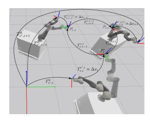
Fig. 3. Transform and frames for three adjacent end-effectors. The transparent manipulators are with desired pose.
