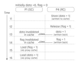
Figure 8. A legal execution on the merged MSI(SC)/RC protocol that adheres to the SC/RC compound memory consistency model. At time t5 a load of flag at P1 reads 1 and at time t6 it correctly reads 1 for data.
