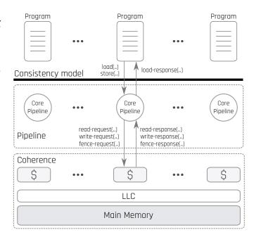
Figure 1. Normally the consistency model enforced by the processor is a function of both the processor pipeline and the coherence protocol combined. We isolate the consistency model enforced by a coherence protocol as the model that is enforced when an in-order pipeline (that issues memory operations one by one) is combined with that coherence protocol.
