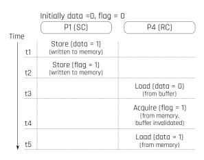
Figure 6. A legal execution on the compound SC/RC machine that adheres to the SC/RC compound memory consistency model. At time t4, an acquire from the RC machine sees flag, at t5 it correctly reads the up-to-date value of 1 from memory.
