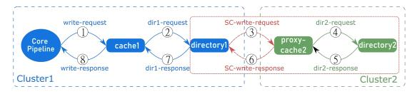
Figure 7. HeteroGen protocol flow for a write issued by the pipeline. Note the red box: directory1, proxy-cache2 and directory2 are one merged directory.
