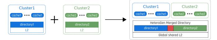
Figure 2. HeteroGen takes as its inputs the coherence protocols of the individual clusters (Cluster1 and Cluster2) and automatically merges their directory controllers to produce the merged directory. The target system model of HeteroGen consists of multiple clusters of cores with their private L1 caches and global shared L2.
